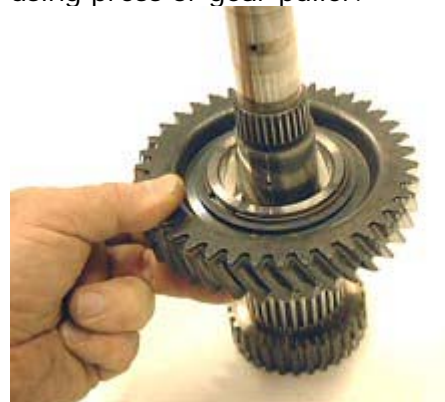
Step 38: Remove low speed gear from main shaft.
