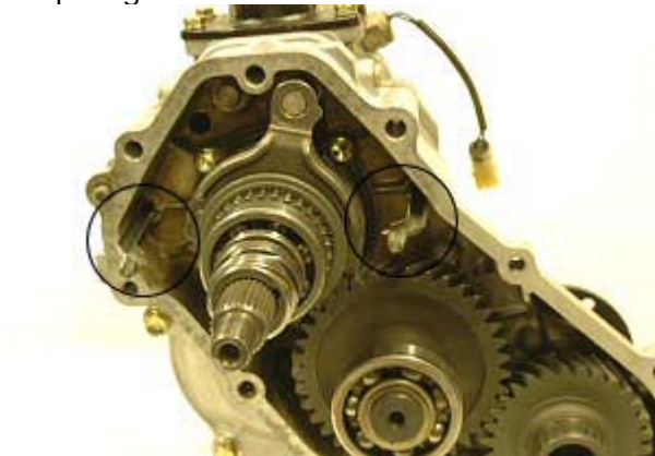
Step 5: Pull out and remove 2 oil transfer tubes.
