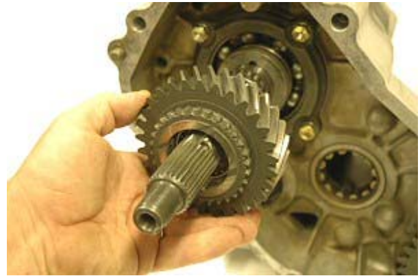
Step 12: Remove front output gear.
