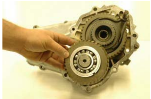
Step 58: Remove counter shaft from cover #1 number and install into cover #2 as shown above.
