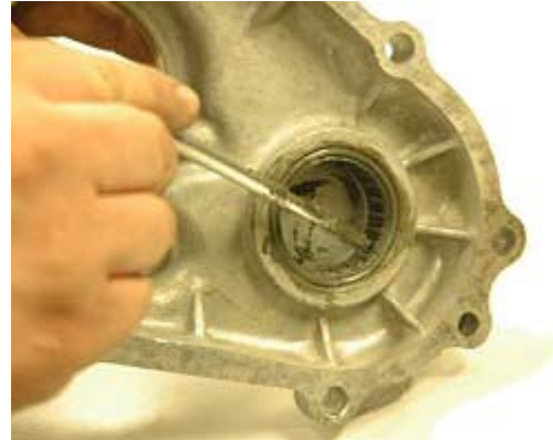
Step 100: Apply grease to cage bearing in rear of cover #3.
