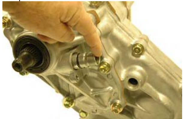
Step 108: Slide speedo drive gear into cover #4.
