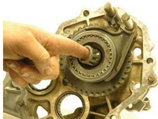
Step 28: Remove pocket bearing from main shaft.
