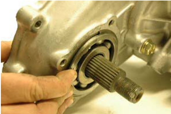
Step 79: Install snap ring around the outside of the front output gear bearing.
