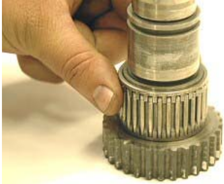
Step 41: Apply grease main shaft race way. Install low speed cage bearing.
