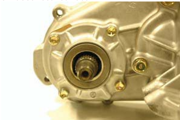
Step 83: Install cover #5 using 4 bolts. Torque to 10 ft/lbs.
