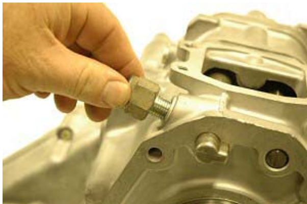
Step 113: Install 4wd shift light switch into cover #1.
