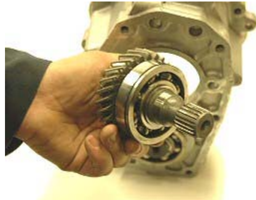
Step 26: Remove input gear.
