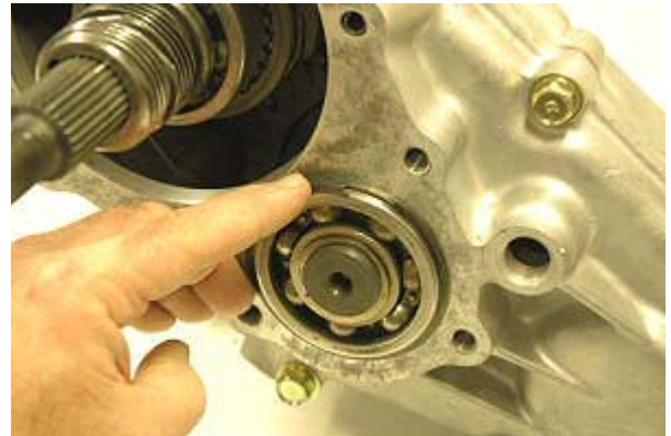
Step 102: Install snap ring onto idler bearing.
