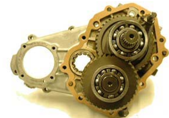
Step 64: Place new gasket onto cover #2.
