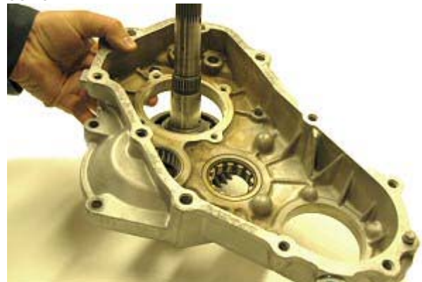
Step 34: Slide cover #2 off of main shaft.
