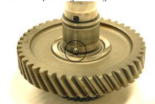
Step 43: Apply grease to the ball hole and insert ball.
