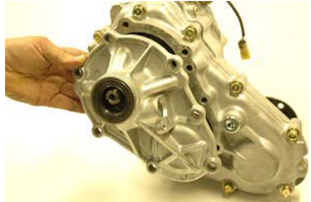
Step 2: Remove 7 bolts and cover #4.
