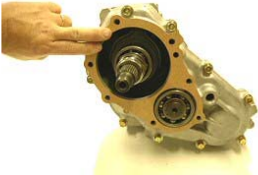
Step 103: Place new gasket onto back of cover #3.
