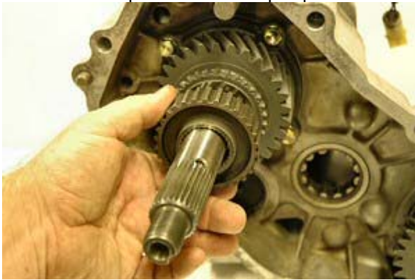
Step 11: Remove front output hub.
