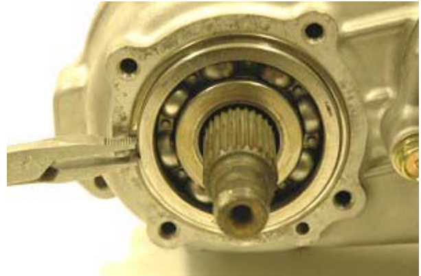
Step 16: Remove front output snap ring.
