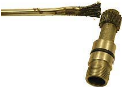
Step 107: Apply grease to speedo drive gear.
