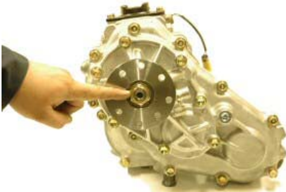
Step 1: Remove 30mm rear nut and flange.
