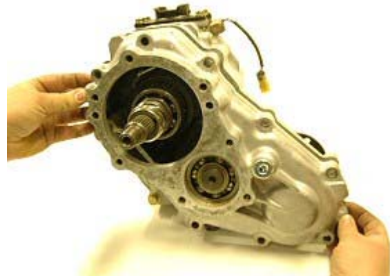
Step 4: Remove 10 bolts and cover #3.
