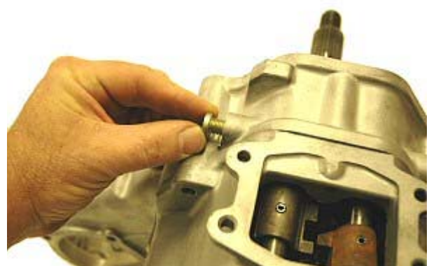
Step 20: Remove detent plug, ball and spring from both sides of upper case. Rotate case on side, then spring and ball will fall out.
