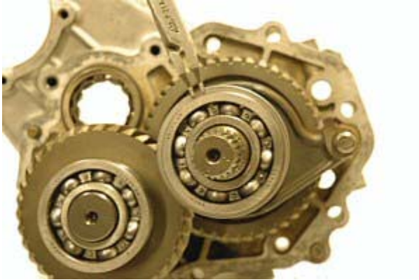
Step 61: Also remove snap ring from input gear bearing.
