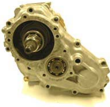
Step 101: Install cover #3 onto the back of cover #2. Be careful to align oil transfer tubes in the cover. Install 10 bolts into cover #3. Torque to 29 ft/lbs.
