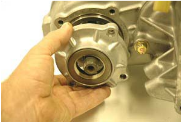
Step 15: Remove front output 30mm nut and flange. Remove 4 bolts. Remove cover #5.
