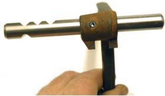
Step 52: Insert roll pin into low range shift fork. Shaft can go in two ways, install as shown above.
