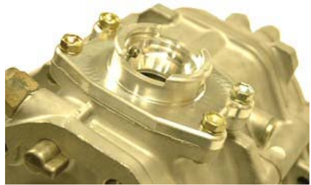
Step 18: Remove 4 bolts, remove shifter base (top shift) or block off-plate (forward shift) depending on model.
