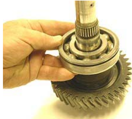
Step 36: Remove 6208N main shaft bearing using press or gear puller.
