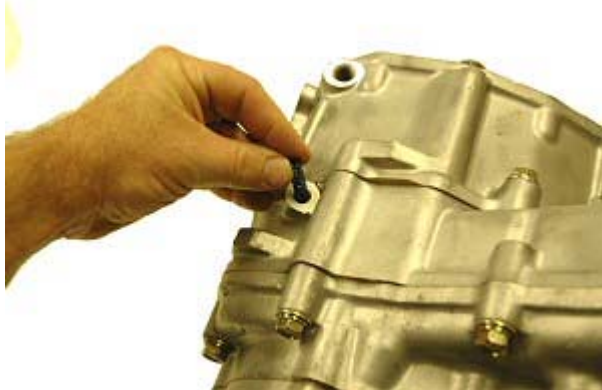
Step 111: Now drop in a detent spring after the ball.
