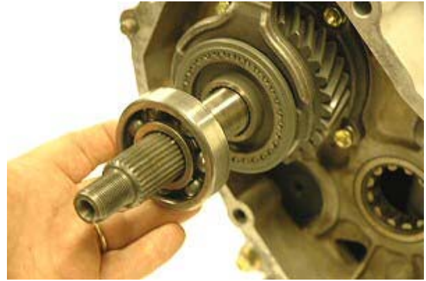
Step 8: Remove 63/28N rear main shaft bearing.
