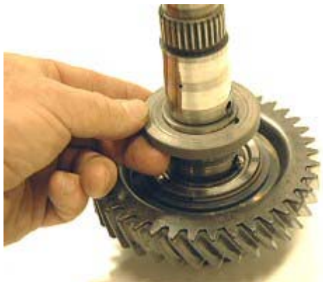
Step 37: Remove thrush washer and lock ball.
