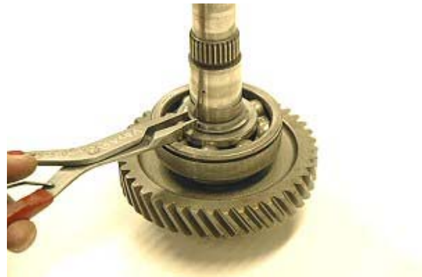
Step 46: Slide 6308N bearing onto main shaft. Press bearing until it contacts thrust washer. Install snap ring onto shaft.
