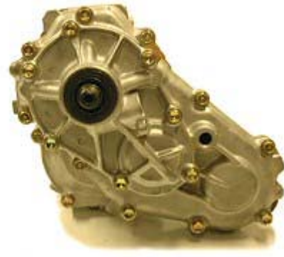
Step 106: Install cover #4 onto the back of cover #3. Install 7 bolts into cover #4. Torque to 29 ft/lbs.
