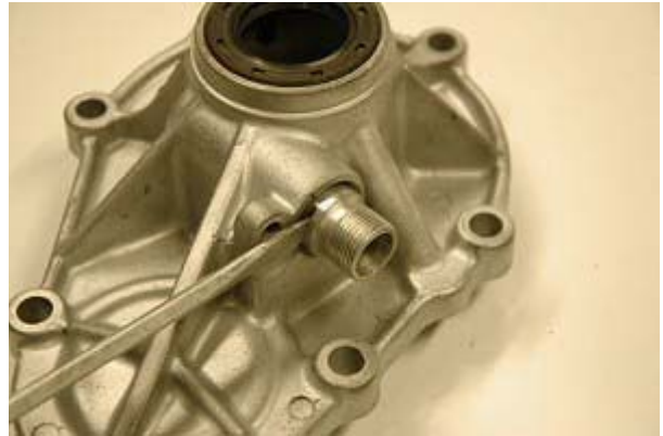
Step 104: Remove speedo lock bolts and tab. Using a screwdriver remove the speedo drive gear from cover #4.
