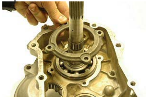
Step 32: Remove 4 bolts and main shaft bearing cover.
