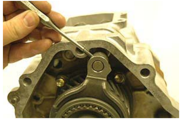
Step 92: Using a 3/16" pin punch, drive roll pin into shift fork so that it is flush with the fork.
