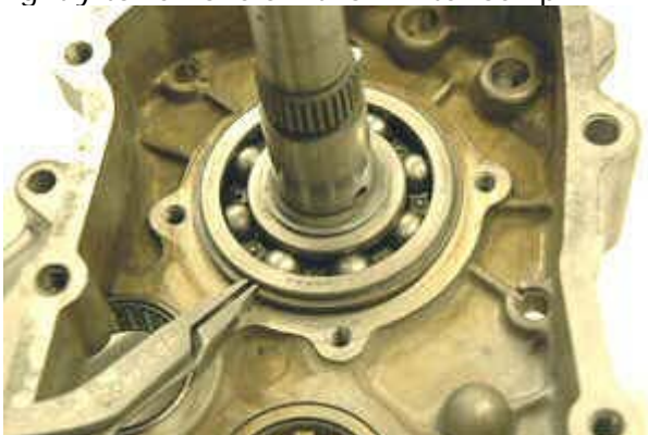
Step 33: Remove main shaft bearing snap ring.
