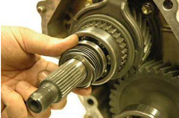
Step 95: Slide oil pump drive gear onto main shaft as shown.
