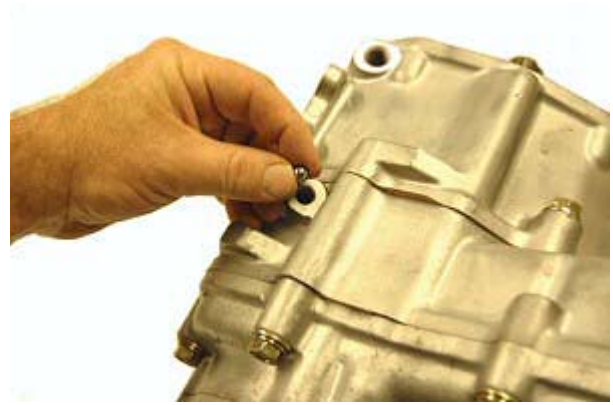
Step 110: With the case on it's side, drop in one detent ball.
