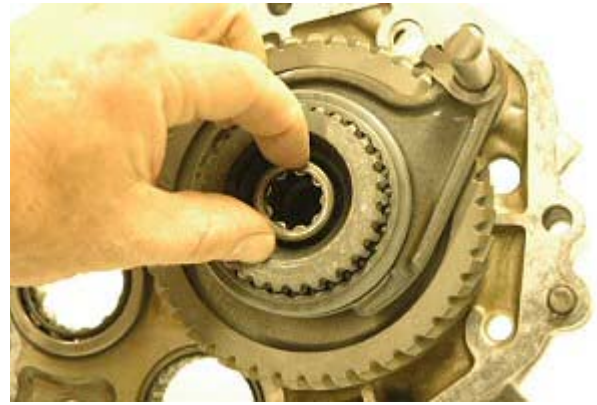
Step 54: Grease pocket bearing inside and out. Insert bearing into main shaft.
