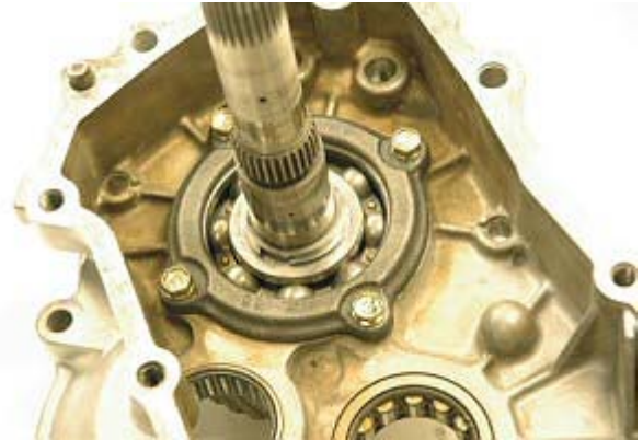
Step 48: Install bearing retainer and 4 bolts. Torque to 10 ft/lbs.
