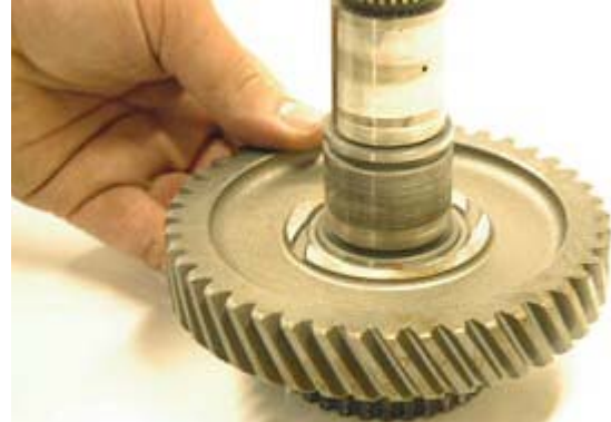
Step 42: Install new 4.70 low speed gear onto main shaft.
