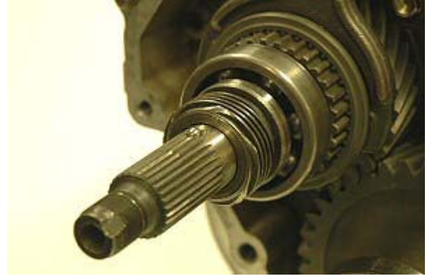
Step 96: Apply grease to ball hole and place ball into hole.
