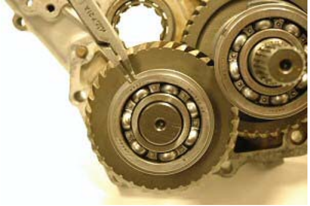
Step 60: Remove snap ring from counter shaft bearing.
