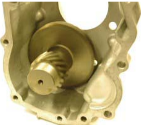
Step 57: Place counter shaft and bearing in cleared housing. Rotate counter shaft to check for proper clearance. Gear should not contact housing when spun.
