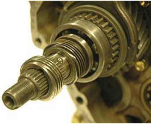
Step 7: Remove speed drive gear, lock ball and oil pump gear. Do not loose ball!
