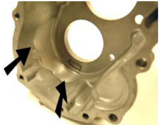
Step 56: Using end mill or hand grinder clearance case as required to accept new 4.70 counter shaft.
