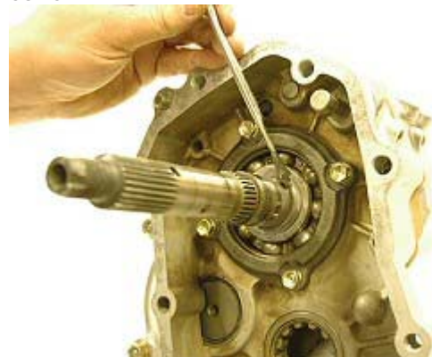
Step 84: Apply grease to ball hole on main shaft and place ball in hole.
