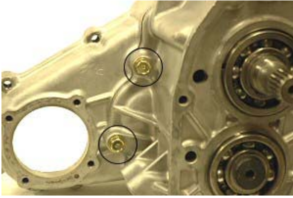
Step 21: Remove remaining 4 bolts holding cover #1. Two bolts are located on the front side, two are on the rear side.
