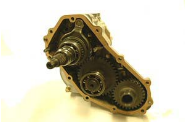
Step 99: Place new gasket onto rear of cover #2.
