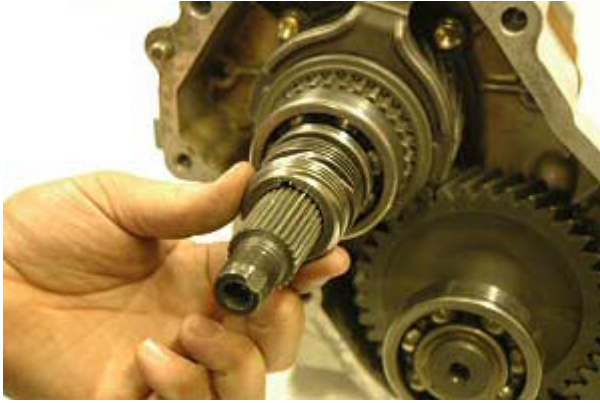
Step 97: Slide speed drive gear onto main shaft.
