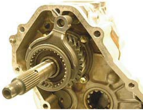
Step 91: Install clutch sleeve and shift fork onto 2wd/4wd shift rail.
