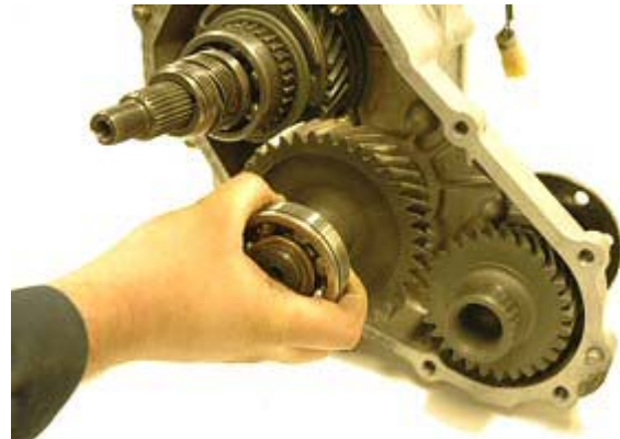
Step 6: Remove front drive idler gear.
