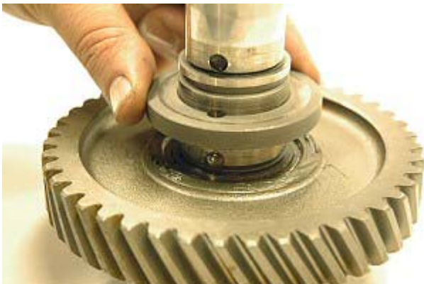
Step 45: Slide thrust washer over main shaft until seated onto face of low speed gear. Line up notch in washer with ball.
