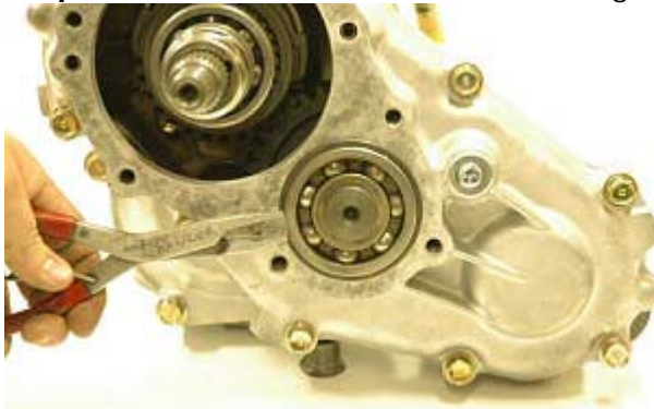
Step 3: Remove 4wd idler shaft bearing outer snap ring.
