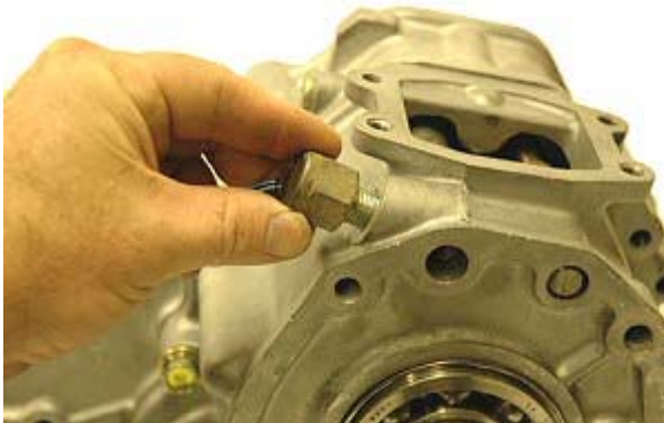
Step 19: Remove 4wd light switch (19mm 1989-1995 or 22mm 1979-1983)
