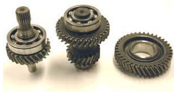
Step 40: Remove snap rings from input and counter shaft gears above. The remaining parts will not be used during reassembly.
