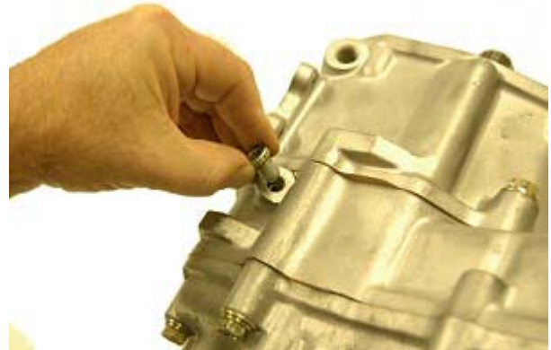
Step 112: Apply silicon to the threads of the detent plug and install. Flip the case over onto the other side and install the ball, spring and plug the same way.
