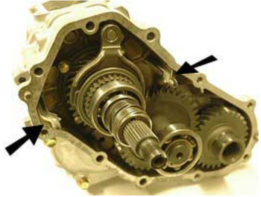
Step 98: Install oil transfer tubes as shown.
