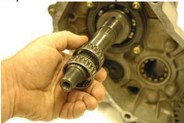
Step 13: Remove (2) 4wd output gear cage bearings.
