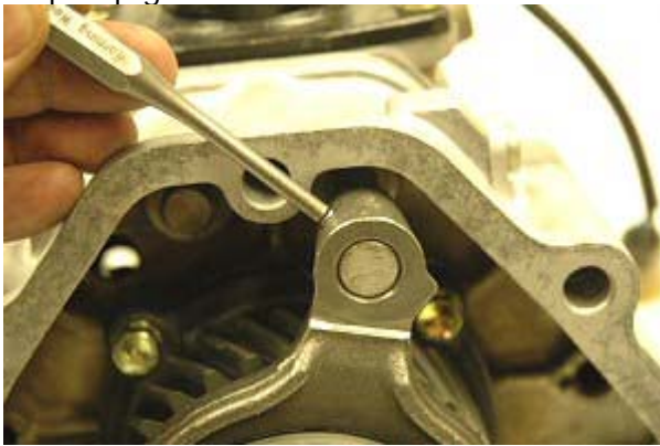
Step 9: Shift into 2wd high. Remove 2wd/4wd shift fork roll pin with 3/16" pin punch.
