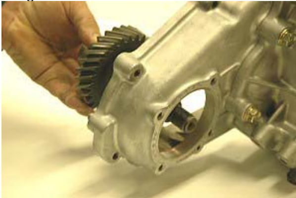
Step 17: Remove front drive output gear.
