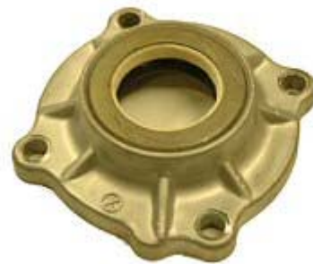
Step 80: Light press front output seal felt and retainer into cover #5.
