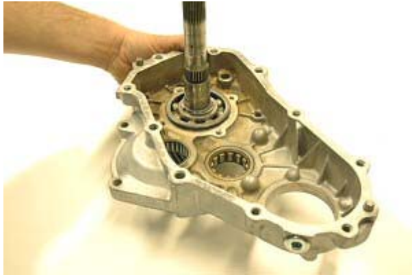
Step 47: Slide cover #2 onto main shaft.
