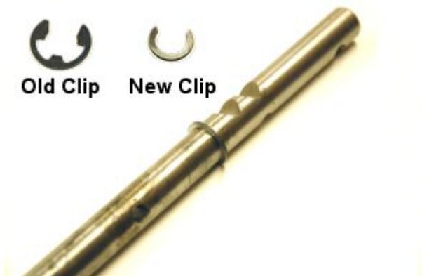
Step 51: On 79-83 models only, replace C-Clip on 2wd/4wd shift fork with new clip provided in kit. Clip is not used on newer cases
