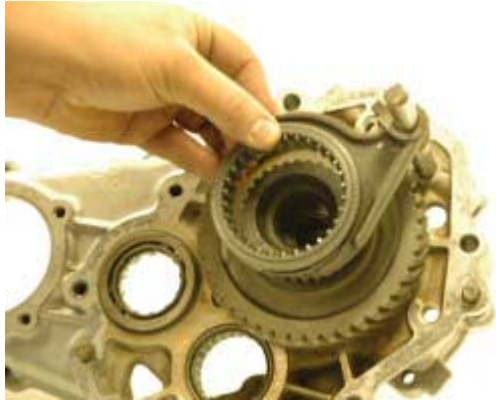
Step 53: Install shift rod, high/low fork and clutch sleeve.
