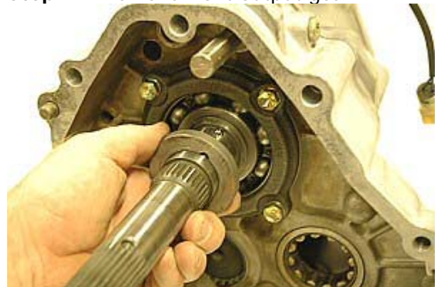
Step 14: Remove thrust washer and it's lock ball.
