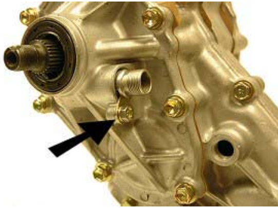
Step 109: Install speedo gear lock bolt and tab, torque to 10 ft/lbs.
