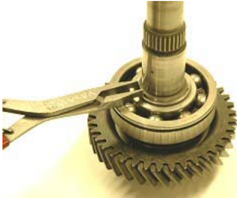
Step 35: Remove snap ring from main shaft.
