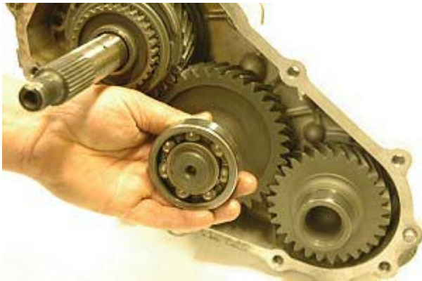
Step 93: Install original front drive idler gear.
