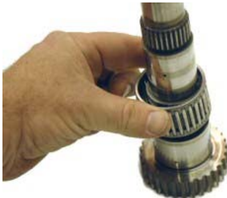
Step 39: Remove main shaft cage bearing.
