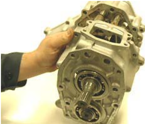
Step 25: Slide cover #1 forward and remove. Retrieve two shift fork roll pins from bottom of housing.
