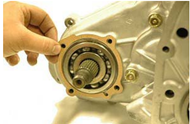
Step 82: Place this gasket onto face of cover #2.
