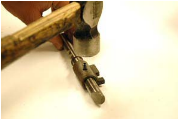
Step 63: 79-83 cases only. Install roll pin into shift block. Note position of shift block fingers and shift rod. Assemble as shown above.
