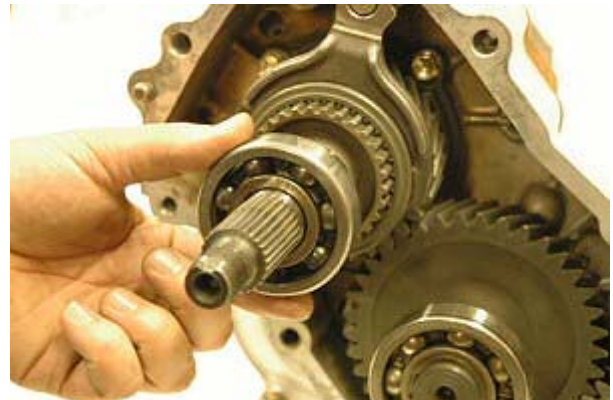
Step 94: Install output shaft rear bearing.
