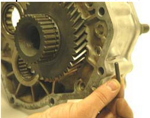
Step 31: Rotate case 90 degrees right, tap case lightly to remove shift fork interlock pin.
