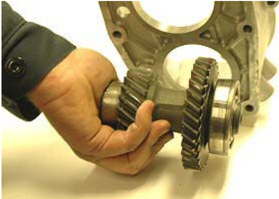
Step 27: Remove counter shaft gear.
