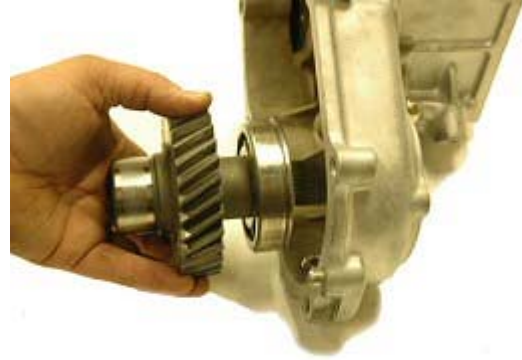
Step 78: Slide front output gear with bearing into cover #2.
