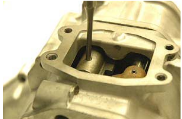
Step 24: Drive out roll pins from both shift rails. Pins will fall to bottom of case.
