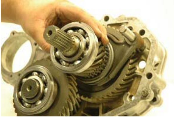
Step 59: Install input gear in main shaft pocket bearing.
