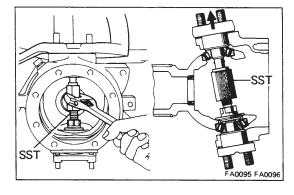
(c) Using SST, push out the knuckle arm and shims from the steering knuckle.
